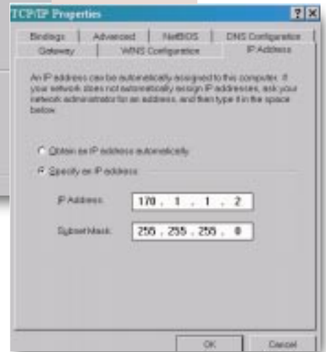
▼ Fig 3 SETTING UP AN IP ADDRESS AND NETMASK
